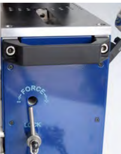
Lever to infinitely adjust the measuring force
