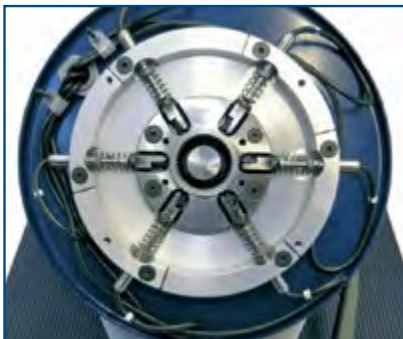
AVM 3x2 RS: 3x2 floating inserts with radius disk
