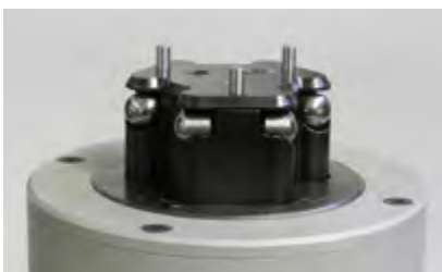
Measuring head with measuring ball inserts and distance bolt
