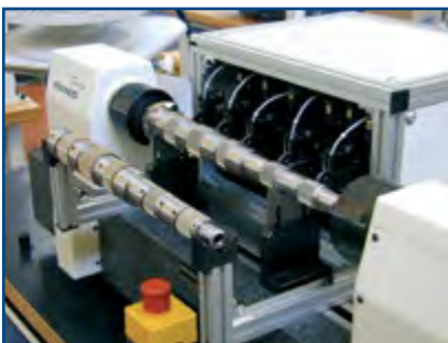
Measurement of a shaft 5 measuring slides for 5 splines with index measurement. Prepared for automatic loading.
