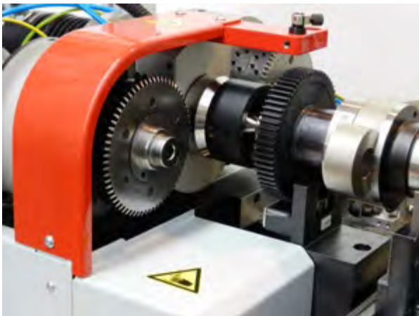
Gear flank analyser with double spindle: cuts measuring time by half
