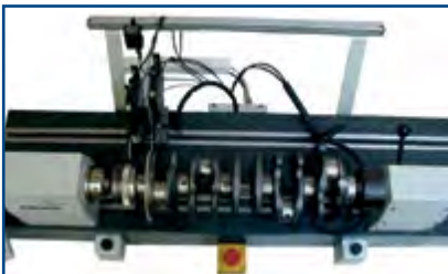
Measurement of a crankshaft Measuring slide for splines.
