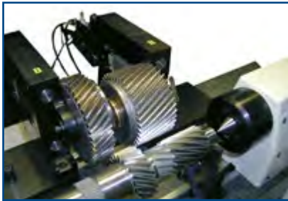
Measurement of splines Double flank gear roll inspection of two gears.
