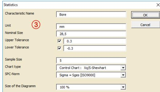
The IBREXDLL allows the statistical analysis of collected measuring data by control charts, run charts, histograms and statistical data in MS-Excel.
